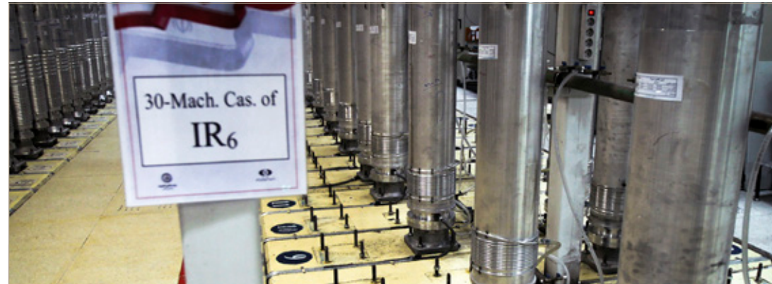
Image: Centrifuges at the Iranian enrichment plant in Natanz.
