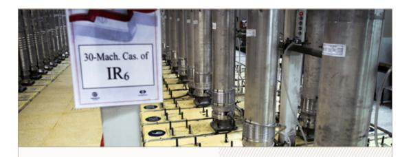
Image: Centrifuges at the Iranian enrichment plant in Natanz.
